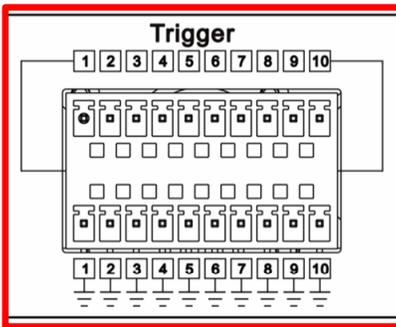
10 Inputs are provided that can be mapped to various functions of the RDM10. The inputs are simple dry contact closures and are provided in ten pairs of trigger and ground connections.
